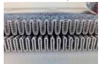
The Filter Media has absorbed water
