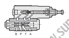
— MRQA is a pressure relief and safety valve with utomatic unloading. Upon reaching the set value, the and ended unloads the pump and puts it under pressure again in the pressure values descend in the circuit to correspond to 65 % or 75% of the set value.
