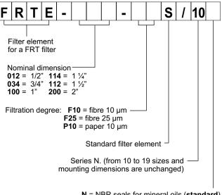
N = NBR seals for mineral oils (standard) V = FPM seals for special fluids (upon request)
