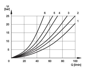
For pressure drops between A and B lines of spools S10, S20, S21, S22 and S23, which are used in the regenerative diagram, refer to curve 5.
