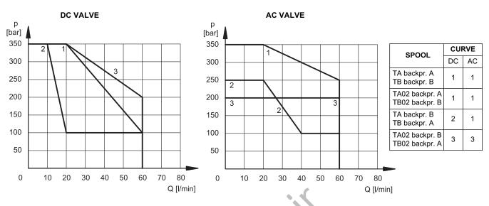
6.3 - AC solenoid valve with coil A110 fed with 110V - 60 Hz
